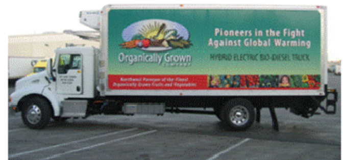
Figure 3: The Kenworth T300 hybrid-electric biodiesel truck
